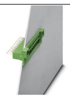
Header, nominal current: 12 A, rated voltage: 320 V, pitch: 5.08 mm, no. of positions: 16, mounting: Direct mounting
